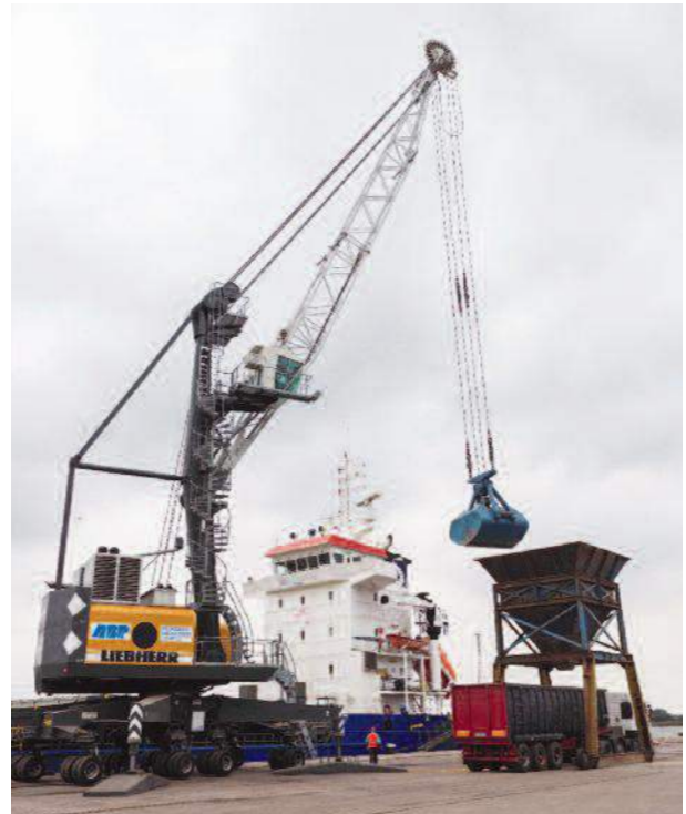
LHM 180 mobile harbour crane with a height of 48.8m at the Port of Newport
